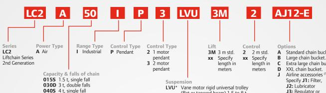
**0405** 4 t, single fall **0605** 6 t, single fall **060Q** 6 t, quadruple falls **080D** 8 t, double falls 120D 12 t, double falls **180t** 18 t, triple falls 250Q 25 t, quadruple falls
